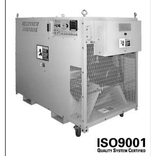
he Avtron Model LPH Load Bank is a portable, self-contained unit that simulates electrical loads. It is ideal for routine load testing of standby diesel generating systems or for factory production line testing of (UPS) Uninterruptible Power Supplies, turbines, or engine generator sets. This model provides resistive loading up to 300 KW at 400 VAC, 50 HZ in a convenient, and easy-to-use package.
